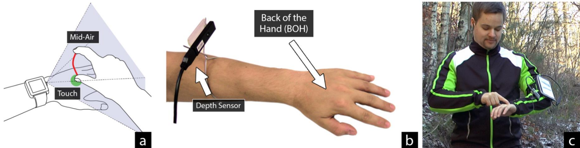
Figure 2. (a) WatchSense enables on- and above-skin input on the back of the hand (BOH) through a wrist-worn depth sensor. (b) Our prototype mimics a smartwatch setup by attaching a small depth camera to the forearm. (c) It tracks the 3D position of fingertips, their identities, and touch on the BOH in real-time on consumer mobile devices. This enables a combination of mid-air and multitouch input for interactive applications on the move [2].
